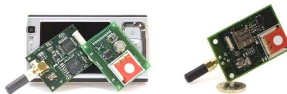
Figure 1. Split- and single-board sensor board designs.
